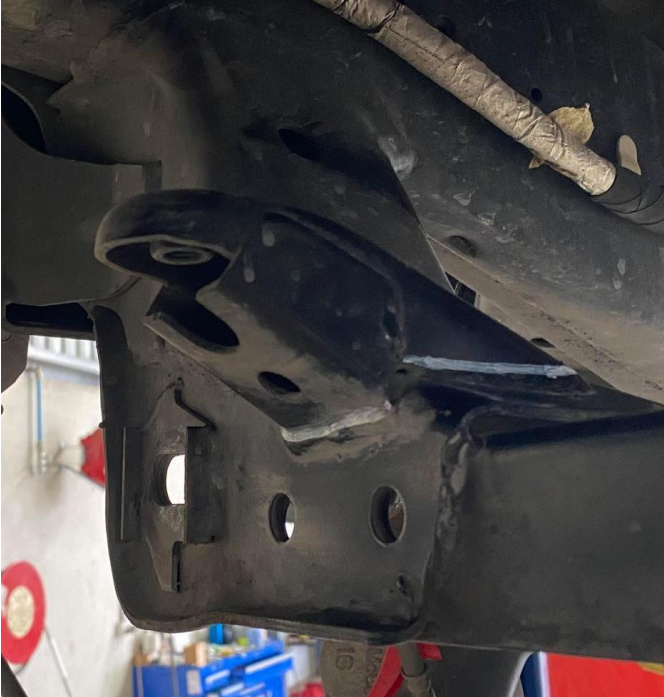
Figure 2: Mark Out Driver Side Diff Mount to Cut
