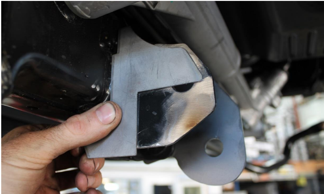
Figure 9: Use Template (PART 7) to Mark for Cutting
