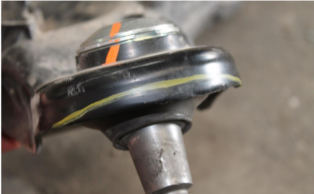
Figure 13: LCA Marked Out to Trim
