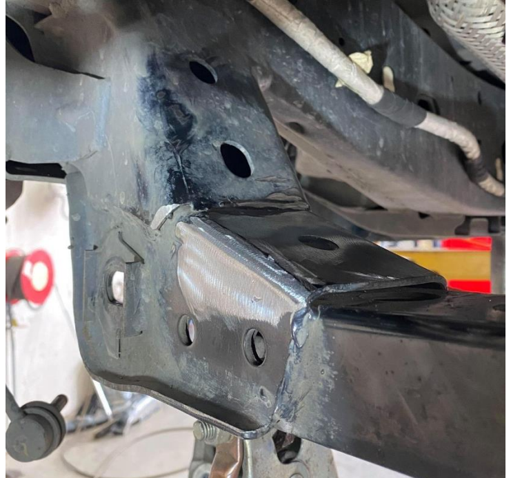
Figure 3: Cut off Diff Mount and grind smooth
